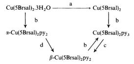
Scheme 1. a, at 105  $^{\circ}$ C; b, over pyridine; c, at 60  $^{\circ}$ C; d, at 80  $^{\circ}$ C.
